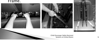
The foam of the bus seat may be depressed to achieve a secure fit and prevent slippage. This will not damage the seat.
