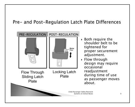
Main difference is use of flow through latch plate (pre) versus locking latch plate (post).
