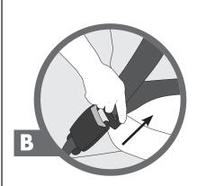
CHECK that the buckle connection is secure by tugging firmly on the seat belt latch plate.
