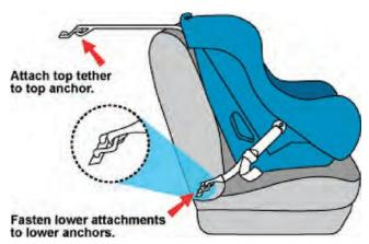
**FIGURE 1**Schematic of the LATCH system.
