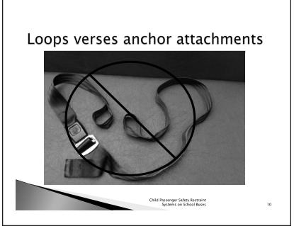
FMVSS 209 gives the requirements for seat belt assemblies. This belt is unacceptable for installation of a CSRS on a school bus because it does not have anchor points meeting FMVSS 209.
