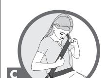
TIGHTEN the lap portion by pulling upward on the shoulder belt. Be sure that the shoulder belt is snug across the chest and crosses the center of the shoulder.
