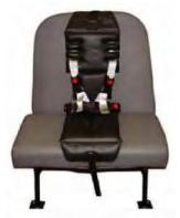
3. Put cushion in place and latch. Under the cushion, bring forward and connect the 1.5" strap to the front side buckle on front of seat (hold the pad on the seat).
